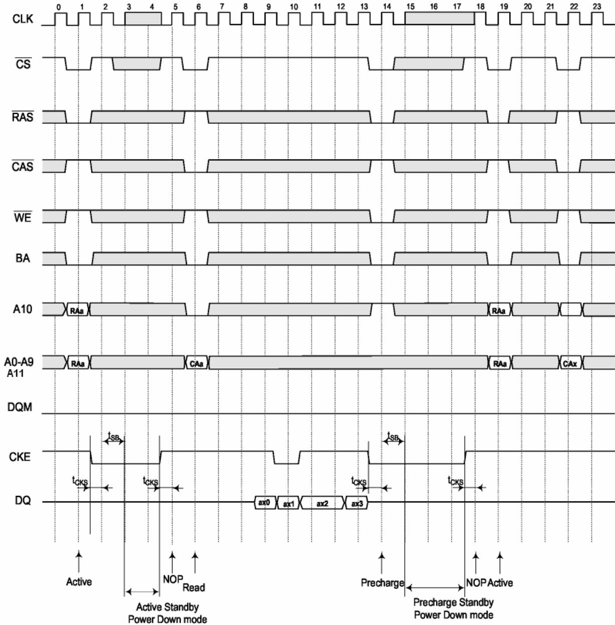
Note: The PowerDown Mode is entered by asserting CKE "low".
