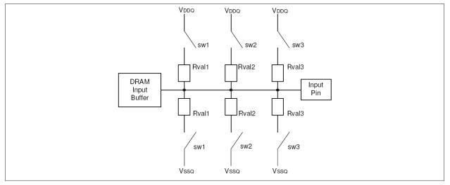
Switch (sw1, sw2, sw3) is enabled by ODT pin. Selection among sw1, sw2, and sw3 is determined by "Rtt (nominal)" in EMR (1). Termination included on all DQs, DM, DQS, DQS pins.
