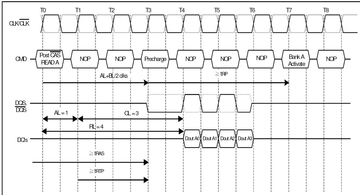
10.17. Burst read operation followed by precharge: RL=4 (AL=1, CL=3, BL=8,  $t_{RTP} \leq 2\text{clks}$ )
