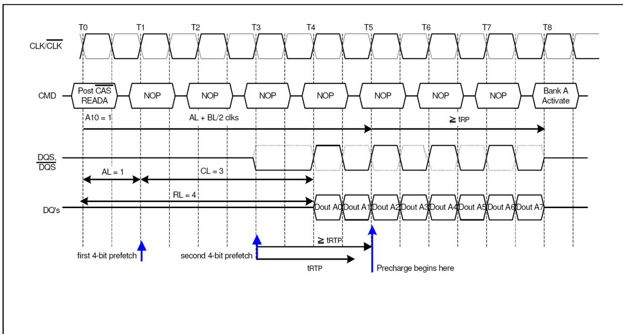
**10.26. Burst read with Auto-precharge followed by an activation to the same bank (tRP Limit): RL=5 (AL=2, CL=3, internal tRCD=3, BL=4, tRTP ≤ 2clks)**
