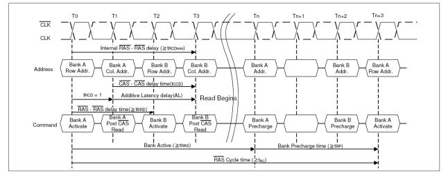
Figure 12 - Bank activate command cycle: tRCD = 3, AL = 2, tRP = 3, tRRD = 2, tCCD = 2
