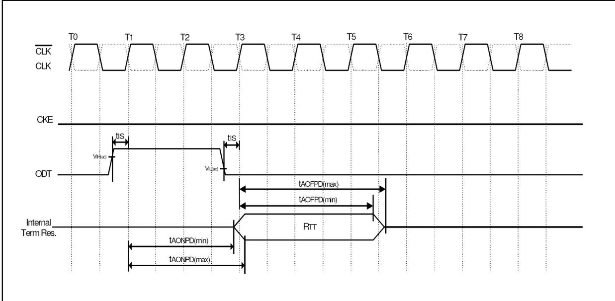
10.5. ODT Timing mode switch at entering power down mode
