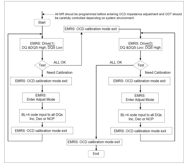
Figure 6 - OCD Impedance Adjustment Flow Chart
