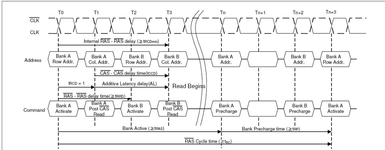
Figure 12 - Bank activate command cycle:  $t_{RCD} = 3$ ,  $AL = 2$ ,  $t_{RP} = 3$ ,  $t_{RRD} = 2$ ,  $t_{CCD} = 2$
