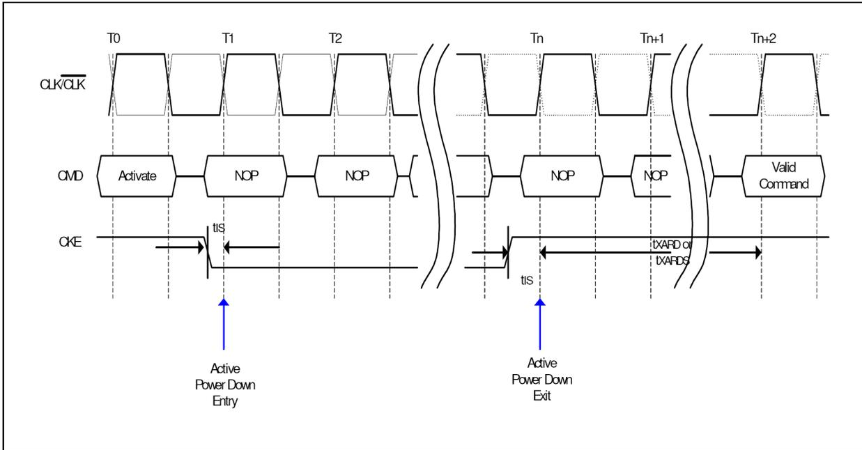
10.31.Precharged Power Down Mode Entry and Exit Timing
