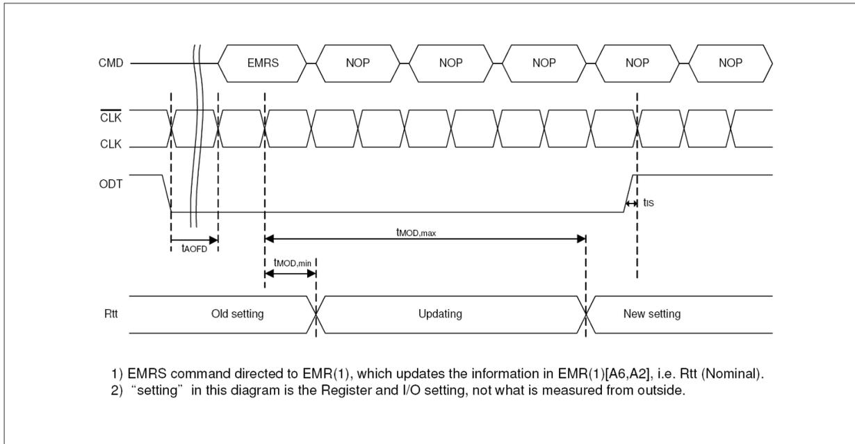
Figure 10 - ODT update delay timing - tMOD
