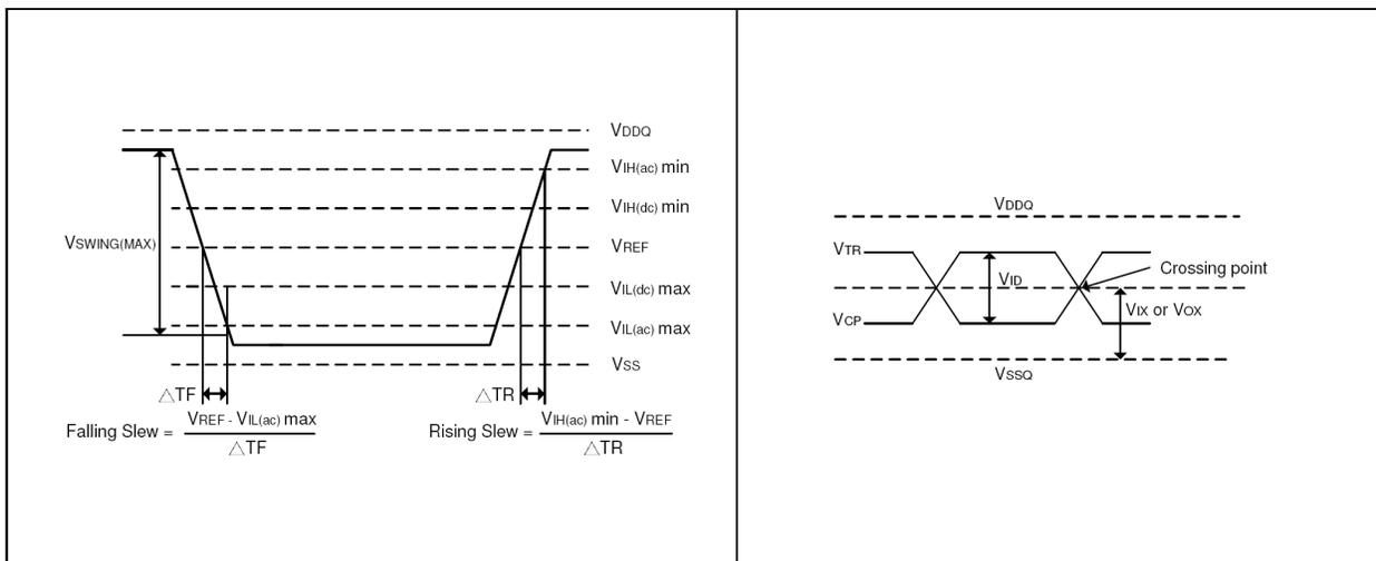
Figure 16 - AC input test signal and Differential input AC signal levels waveform
