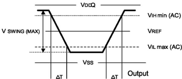
$$SLEW = (V_{IHmin} (AC) - V_{ILmax} (AC)) / T$$
