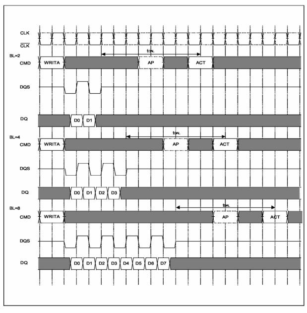
The Write with Auto Precharge command cannot be interrupted by any other command. AP Represents the start of internal precharging .
