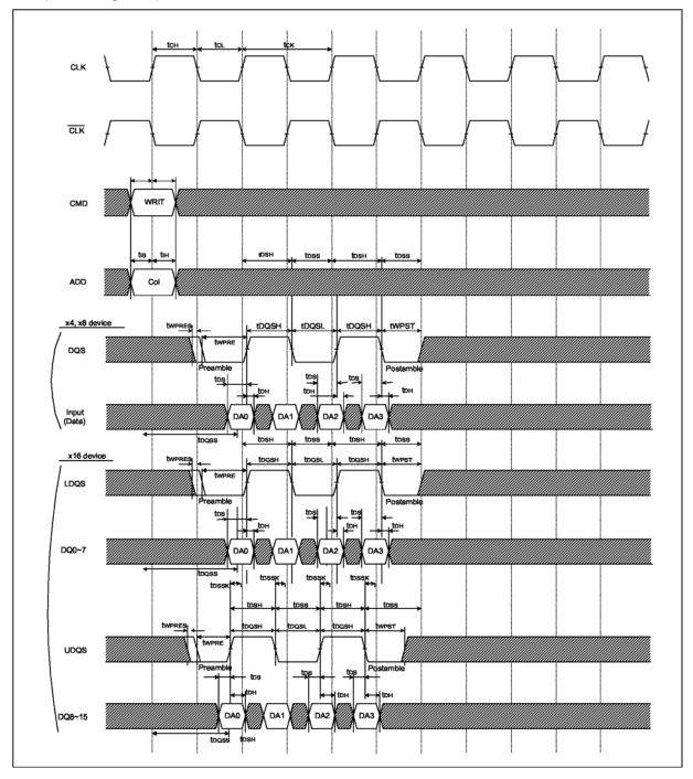
**Note:** x16 has 2DQS's (UDQS for upper byte and LDQS for lower byte). Even if one of the 2 bytes is not used, both UDQS and LDQS must be toggled.
