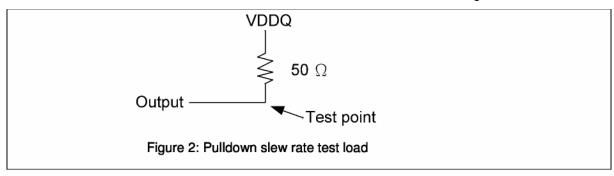
c. Pullup slew rate is measured between (VDDQ/2 - 320 mV  $\pm$  250 mV) Pulldown slew rate is measured between (VDDQ/2 + 320 mV  $\pm$  250 mV) Pullup and Pulldown slew rate conditions are to be met for any pattern of data, including all outputs switching and only one output switching.
