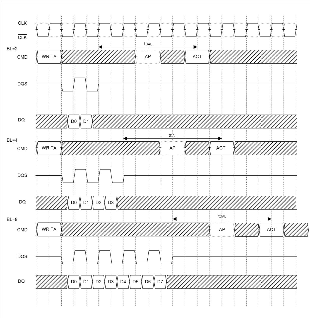
The Write with Auto Precharge command cannot be interrupted by any other command.
