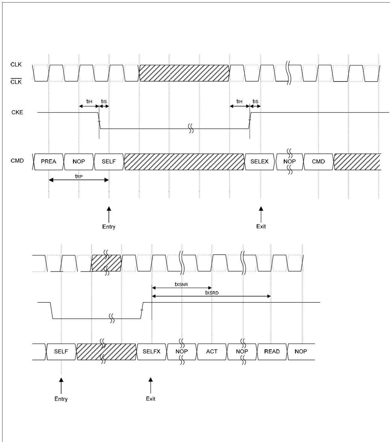
**Note:** If the clock frequency is changed during self refresh mode, a DLL reset is required upon exit.
