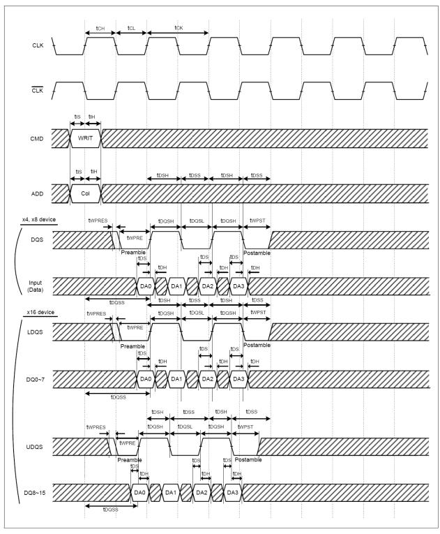
**Note:** x16 has 2DQS's (UDQS for upper byte and LDQS for lower byte). Even if one of the 2 bytes is not used, both UDQS and LDQS must be toggled.
